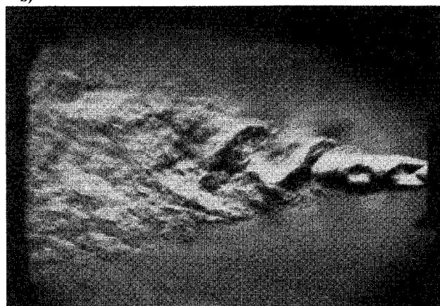
Fig. 18 Schlieren photographs of the underexpanded jets: a) circular jet; b) elliptic jet—major, 5 ns exposure; c) elliptic jet—minor, 5 ns exposure.
